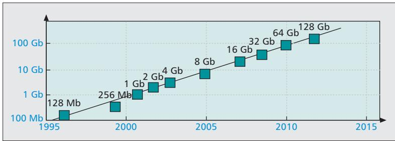
**Figure 1.** The market introduction of single-chip flash memory capacity showing a doubling in capacity every 18 months along Moore's Law, leading to a  $10\times$  increase every five years.
