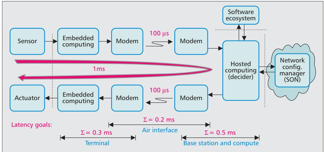
Figure 4. The impact of breaking down the 1 ms round-trip delay.
