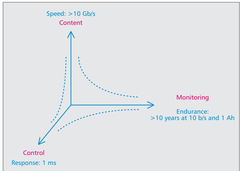
**Figure 5.** The wireless network moving from communications of content to monitoring to control. The dashed lines indicate that applications allow for a trade-off between the three depicted criteria of optimization: speed, response time, and operation endurance.
